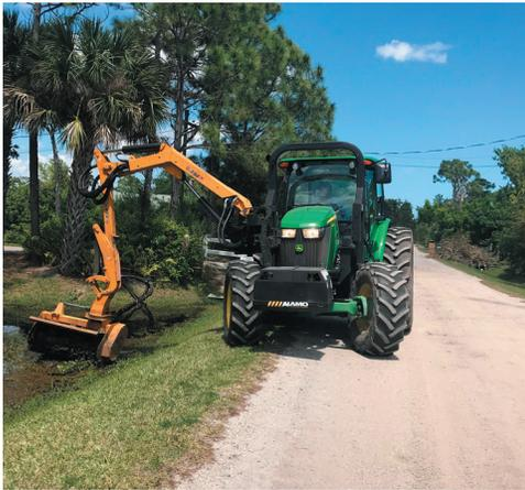
clean the slopes of our Town's drainage ditches. The John Deere tractor can also support several other attachments. One of those attachments is the Alamo Boom Ditcher. This attachment is like a snow blower for ditches. It scoops the dirt from the bottom of the ditch and ejects it through a chute at the top. This piece of equipment has been used to great effect on many of our Town's roads, such as Elaine Ln., Duncil Ln. and Kelly Ln.
